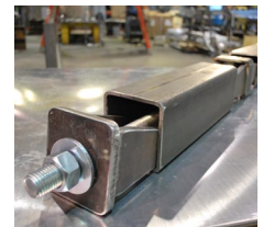
Demonstration model shows bolt-up hardware.
